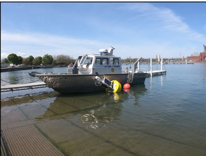
The new GLOS buoy being prepared for deployment. The newer buoy is smaller and lighter, and is made from hard foam instead of fiberglass.
