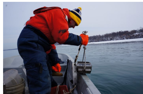
Graduate student Anthony is about to launch his first Ponar grab at the lower Niagara River in March 2015.
