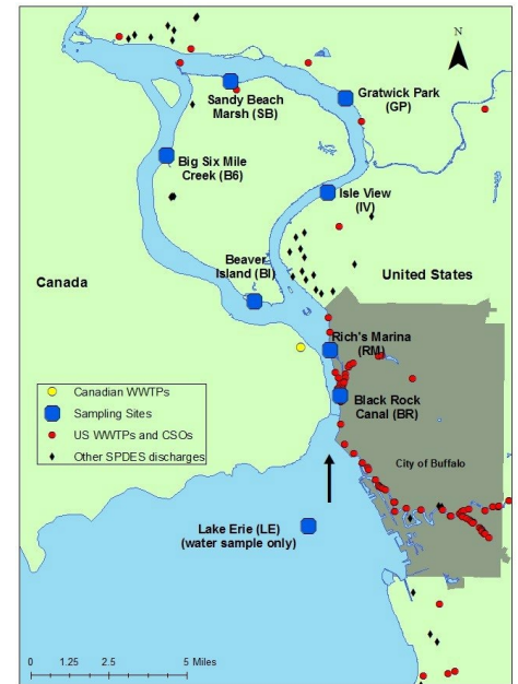
Map of my sampling sites, which also shows the location of combined sewer overflow discharge points, and non-sewage discharges from industrial sources (State Pollutant Discharge Elimination System, or SPDES). Lake Erie water samples were taken as a reference for E. coli observations.
