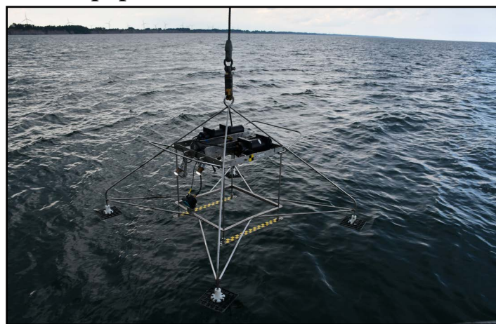
The Benthic Imaging System (BIS) is a drop-down frame with down- and side-looking cameras and lights.
