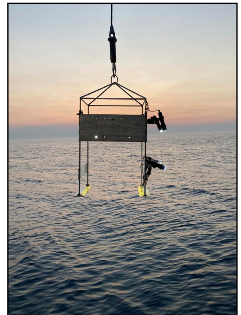
The Benthic Imaging System, which has downward and sideways pointing cameras and lights, being lowered into
