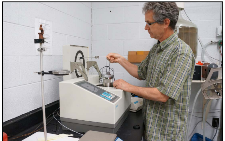
Mark Clapsadl using a calorimeter to determine the energy content of emerald shiners. Calorimetry was also used for the preservation methods study.
