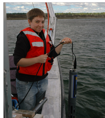
Kit deploying the YSI to sample a profile.
