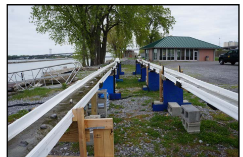
Two raceways used for growing algae.
