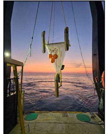
Benthic sled being deployed.
