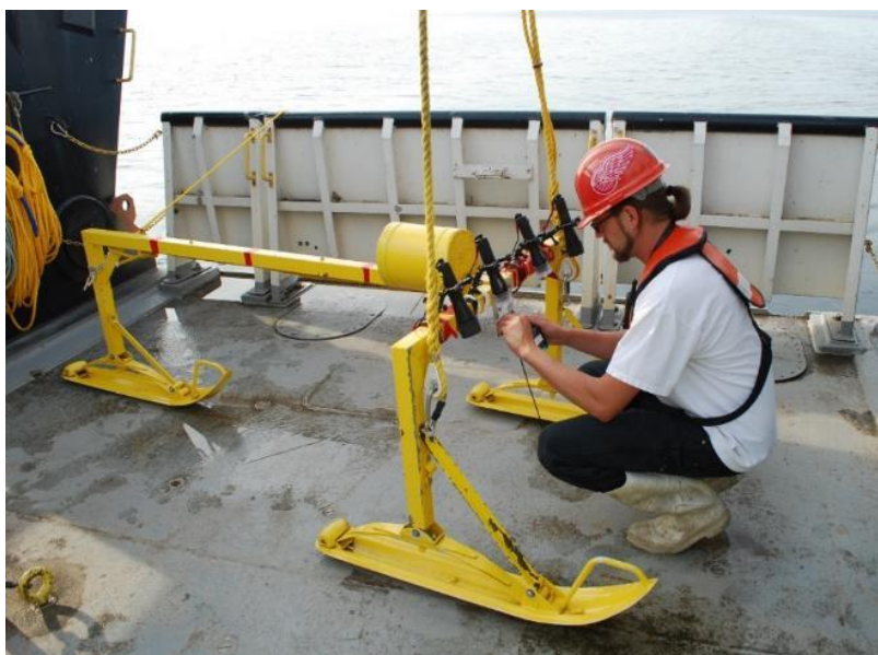
Figure 2.2. R/V Lake Guardian marine technician Maxwell Morgan attaching GoPro camera to the benthic sled during the Lake Huron CSMI benthic survey in 2017.
