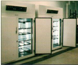
Environmental chambers used for growing aquatic plants and algae.
