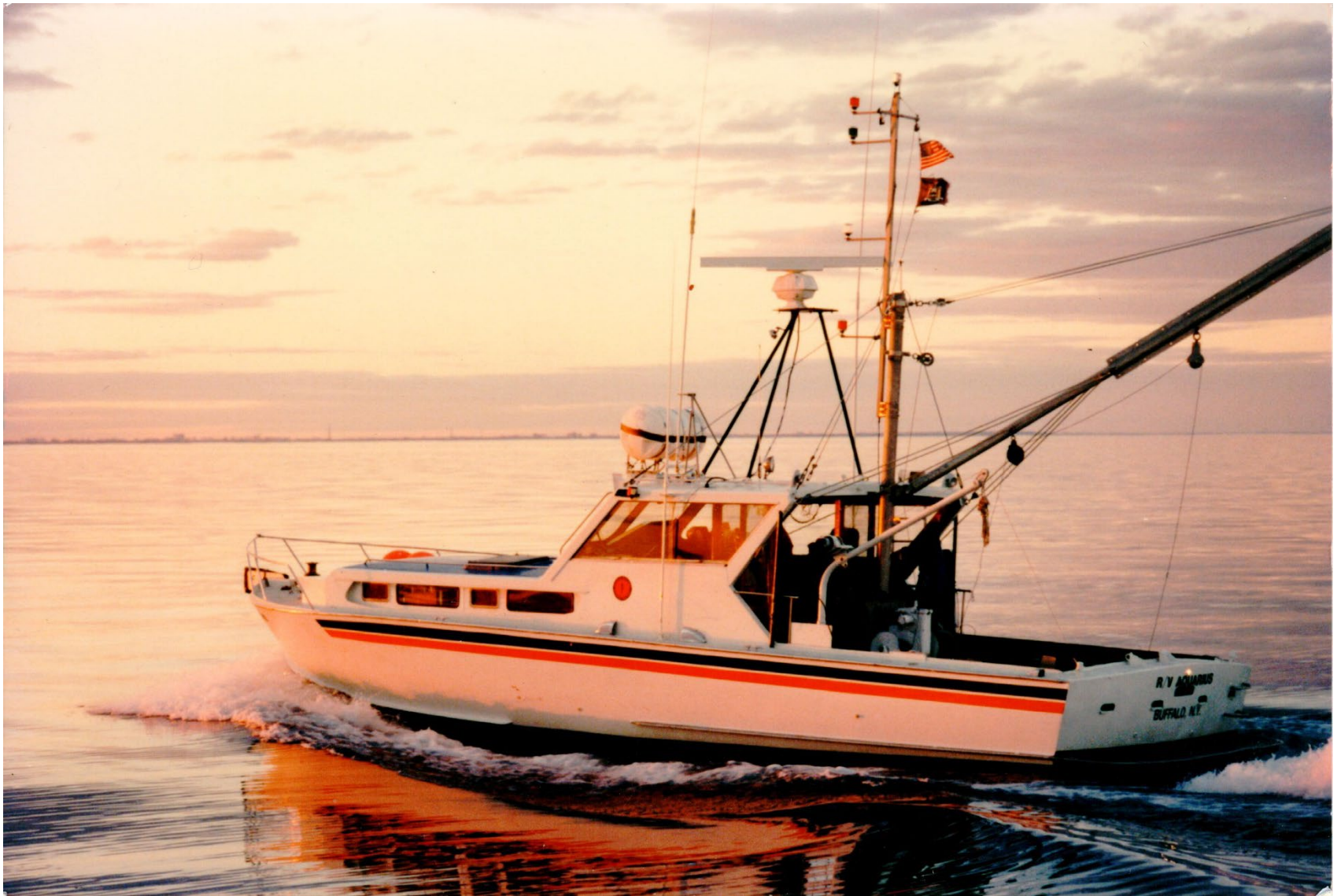
R/V Aquarius, 40' steel-hulled vessel used from 1996 through mid-2000s
