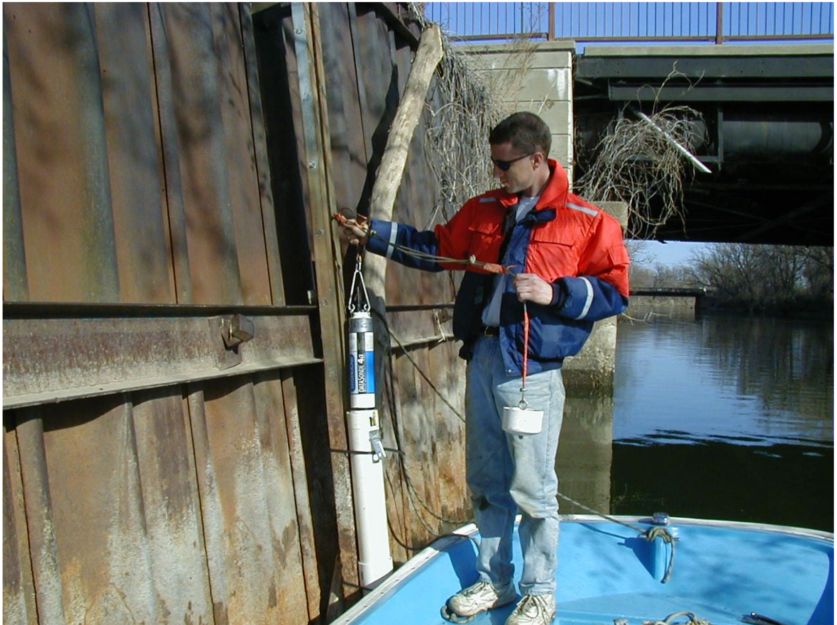
Installing Hydrolabs for the CSO project
