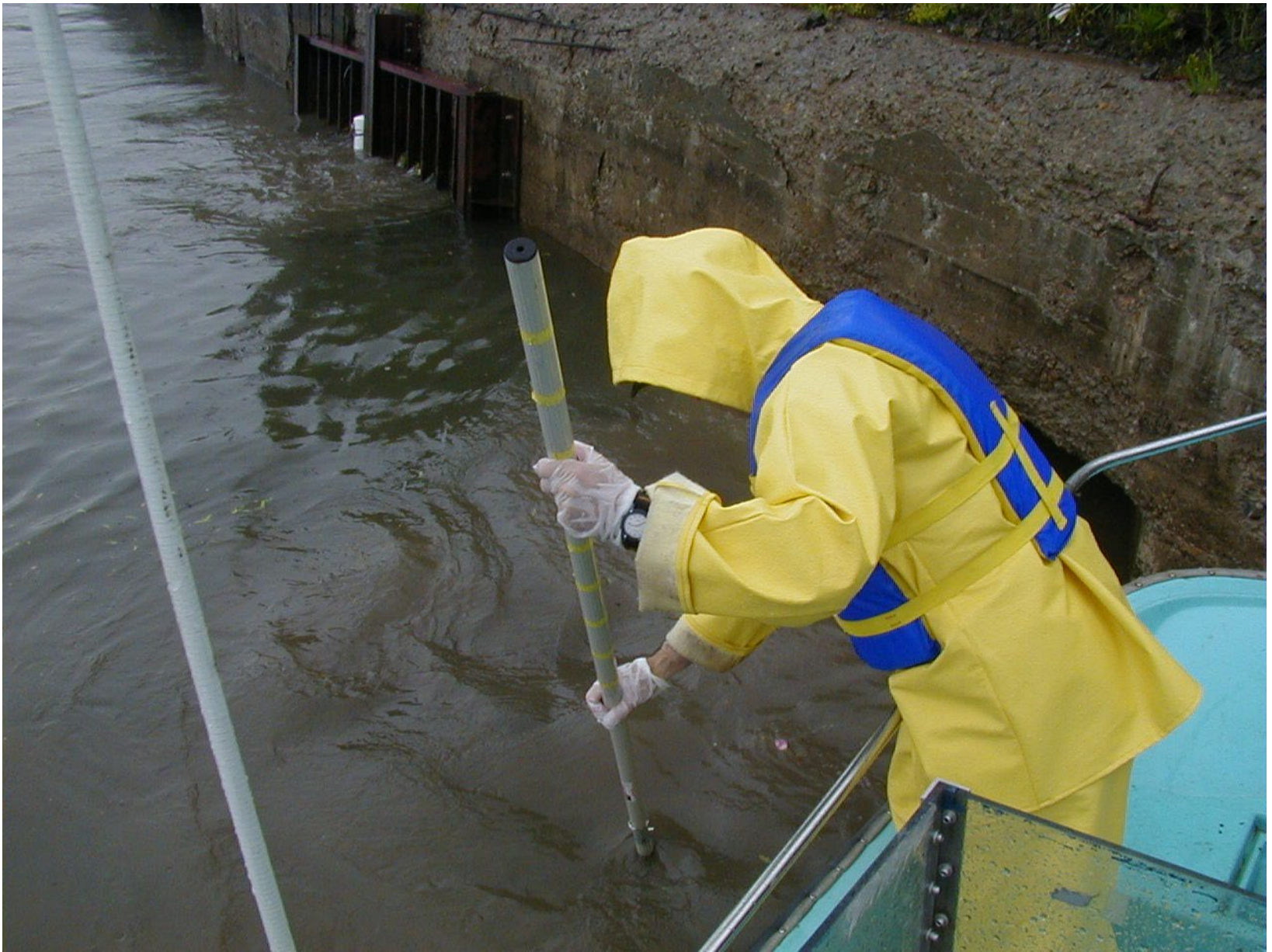
Combined sewer overflow sampling
