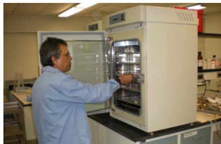
Jagat Mukherjee with different cell lines (including cancer cell lines) that are being incubated at controlled temperature and an atmosphere of 5% carbon dioxide.
